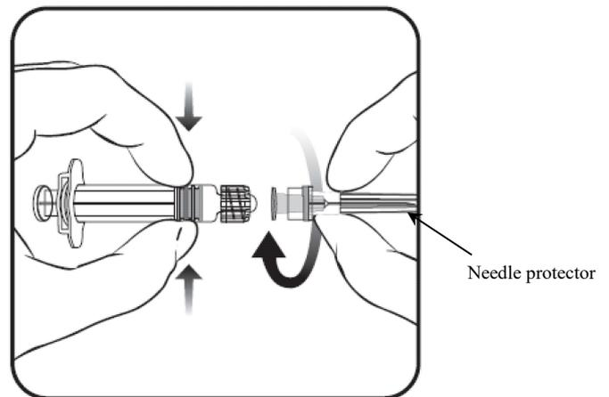
4. Add the solvent to the powder. After the addition of the solvent to the powder, the mixture should be well shaken until the powder is completely dissolved in the solvent.
